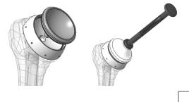
Place selected Adapter Ring onto the Humeral Tray. Reduce shoulder and perform final functional evaluation. Confirm final implant placement fluoroscopically or radiographically.
